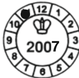
The Finnish re-verification mark. In this example the re-verification is carried out in November 2007.
