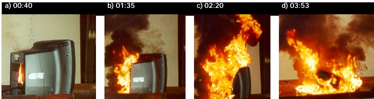
Picture 2. A series of pictures of burning tests for television sets.
